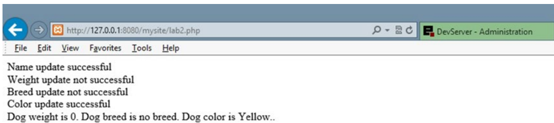
Figure 3-3. Output with invalid weight (1000) and invalid breed ('Lab12') in Dog class— dog.php and lab.php
