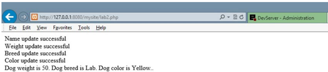
Figure 3-2. Output of successful update via set methods in Dog class— dog.php and lab.php
