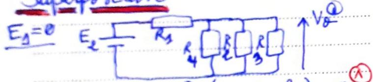
Voltage divider  $\Rightarrow V_o^{(1)} = \frac{(R_2 \parallel R_3 \parallel R_4) E_2}{(R_2 \parallel R_3 \parallel R_4) + R_1}$
