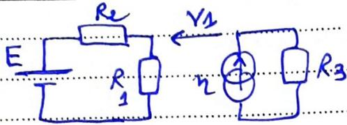
$$V_1 = \frac{R_1}{R_1 + R_2} E - R_3 \eta \quad (\text{A})$$
