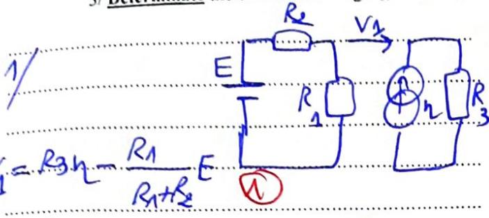
$$V_1 = R_3 \eta = \frac{R_1}{R_1 + R_2} E$$
